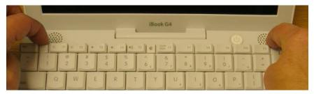
1. Use your index fingers to pull the two tabs down toward you and carefully lift up the top of the keyboard.
